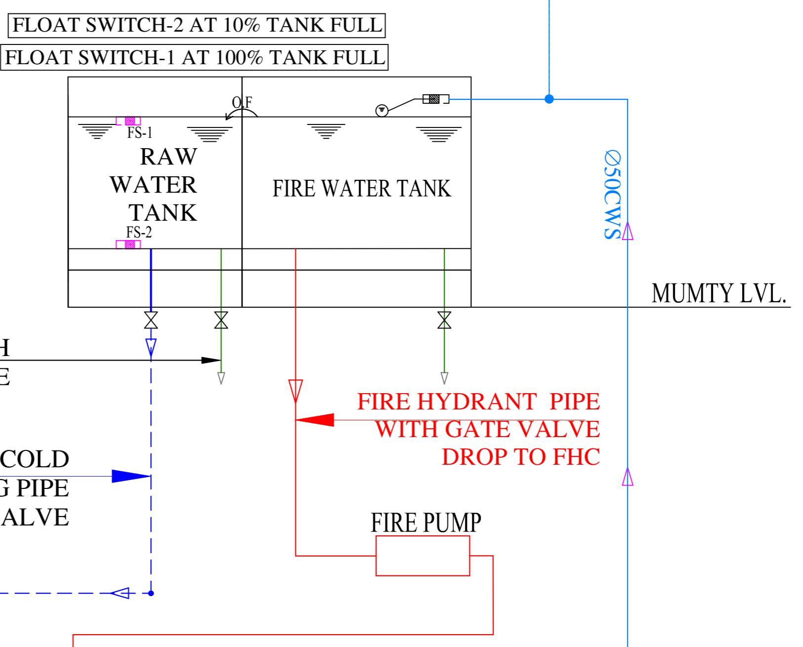
50MM DIA OVER HEAD RAW WATER TANK FILLING LINE
