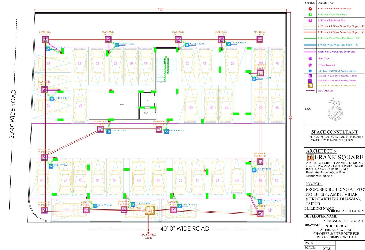
Ø110 mm Soil Waste Water Pipe Ø110 mm Waste Water Pipe Ø110 mm Rain Water Pipe Ø 160 mm Soil Waste Water Pipe Slope 1:150 **Ø**110 mm Soil Waste Water Pipe Slope 1:150 **Ø**110 mm Waste Water Pipe Slope 1:150 **Ø**75 mm Waste Water Pipe Slope 1:150 50mm Waste Water Pipe Bottle Trap Gully Trap-12"X12" Depth Acording to Slope Main Hole-18"X18" Depth According to Slope Main Hole-36"X32" Depth Acording to Slope
