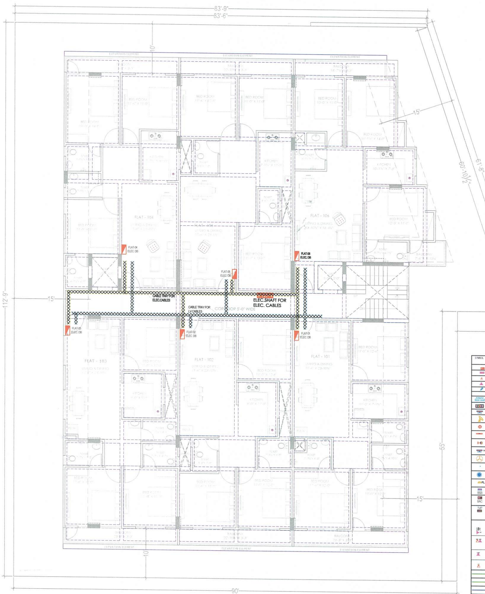
TYPICAL FLOOR (G+5) ELECTRICAL ROUTE LAYOUT
