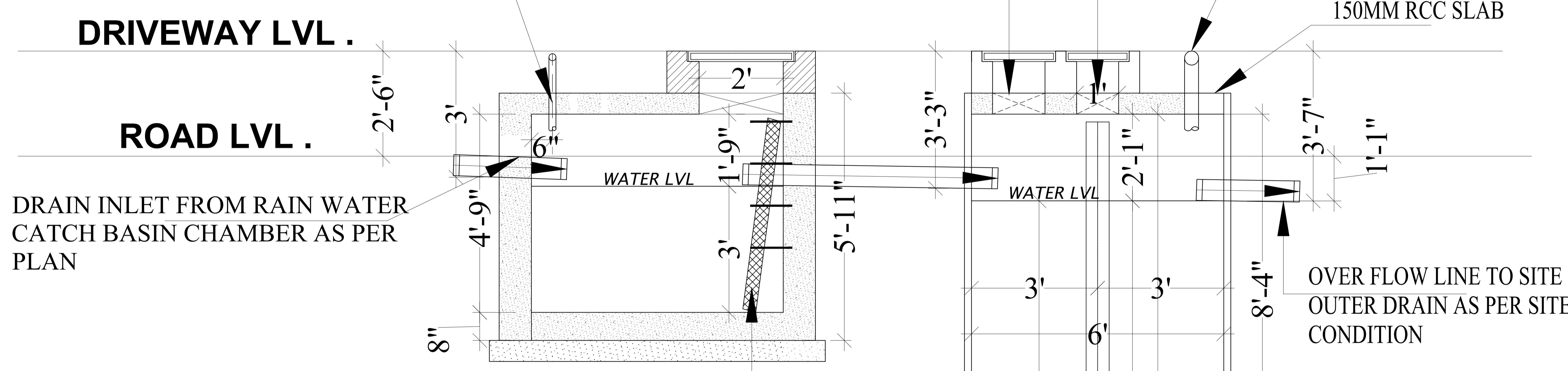
GRATING OF MIN. SIZE WITH 16 mm SQ. BARS & FRAME @ 20 mm CLEAR SPACING FIXED AT THE MOUTH OF PIPE AS PER SITE CONDITION
